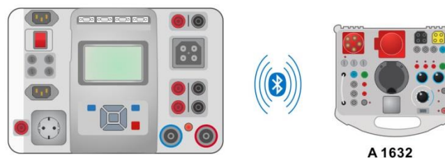
Figure 8.5: Connection of the eMobility Analyser (A 1632)
