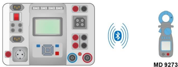
Figure 8.6: Connection of Leakage clamp meter with Bluetooth® communication
