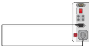
Figure 6.139: Polarity test (manual)
