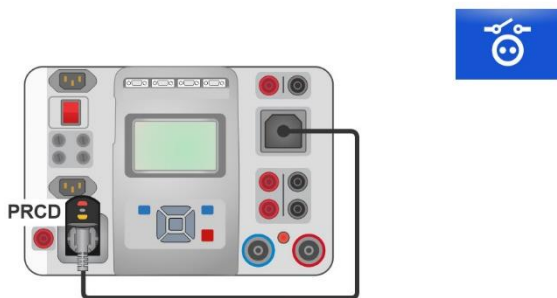
Figure 6.125: Connecting portable RCDs (PRCDs)
