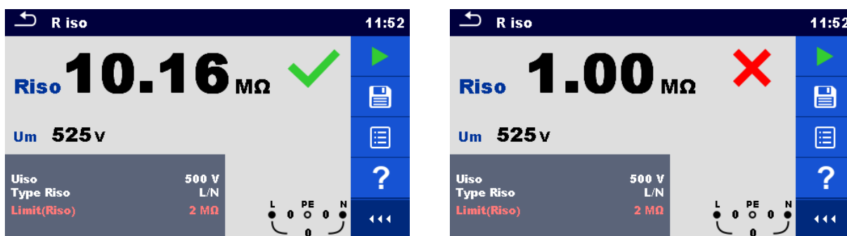
Figure 6.32: Examples of Insulation resistance (Installations) measurement result
