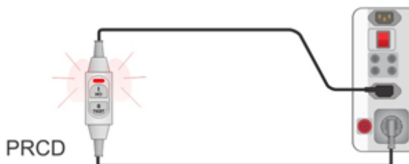
Figure 6.118: PE conductor (PRCD) test
