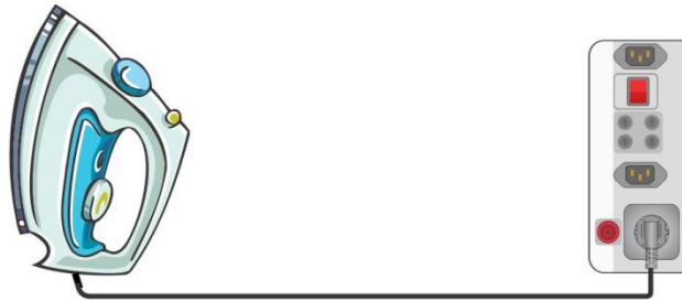
Figure 6.25: Insulation resistance Riso (socket)
