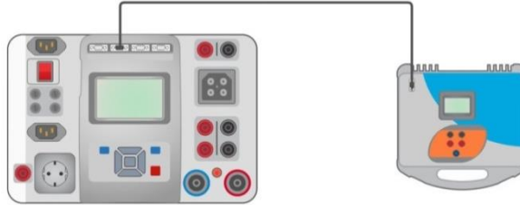
Figure 8.3: Connection of the Euro Z 290 A adapter A 1143
