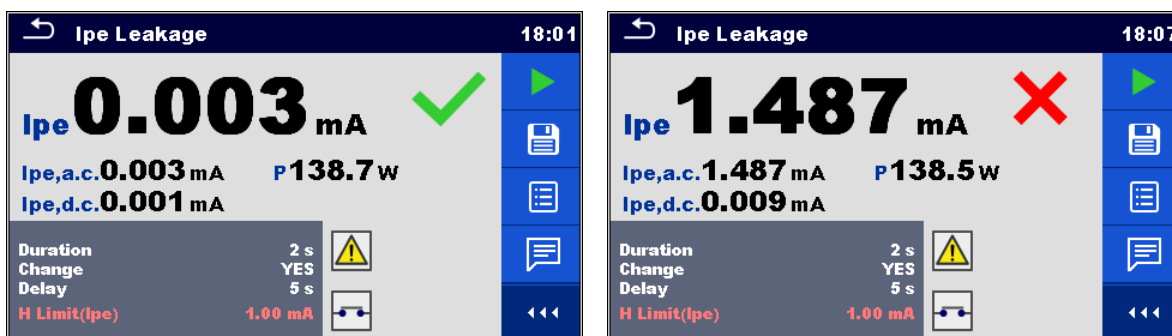
Figure 6.46: Examples of I pe Leakage measurement results
