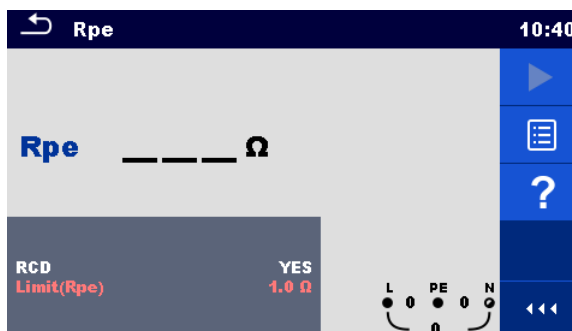
Figure 6.107: PE conductor resistance measurement menu
