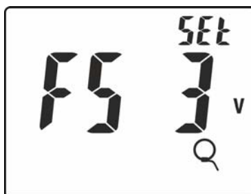
Fig. 7: Setting full scale of flexible clamp
