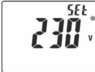
Fig. 6: Setting the rated voltage in Loop measurement
